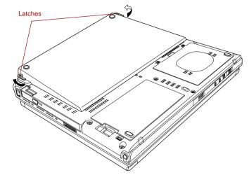
Figure 6-6 Releasing the latches
